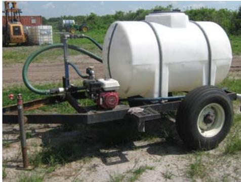
Figure 1. Example of a large nurse tank for mixing SoilGard in water for injection into a drip irrigation system. Note the recirculating pump (lower left) for mixing to keep the product suspended in water.
