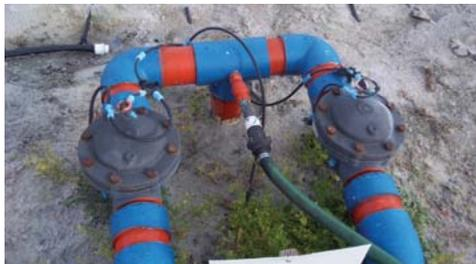
Figure 2. Injection point with hose coming from the nurse tank in Figure 1.
